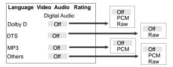
When using the coaxial cable(see page9), you should set Digital Out PCM or Raw. Refer to the amplifier's owner's manual and make the setting Raw or PCM. Select one mode, if there is no sound change to the other one.
